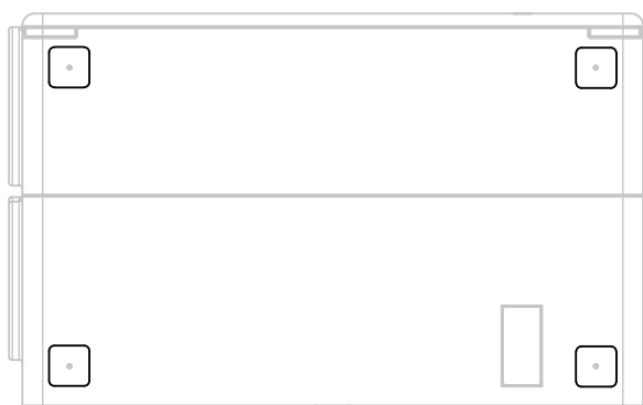
Bonding points of the mounting feet for heat recovery unit standing horizontally in the standard version
